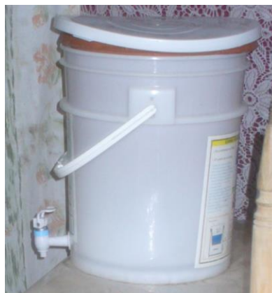
Figure S-1 Photo of a distorted lid that does not adequately cover the filter.
