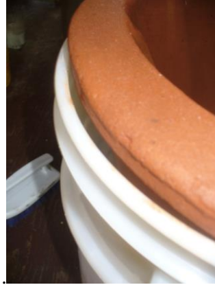
Figure S-2 Photo of manufacturing defect in filter.
